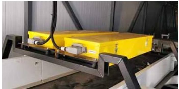
PI-MSKA system mounted above belt conveyors
