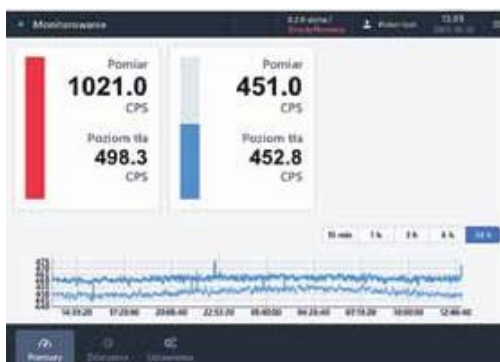
Monitoring with triggered alarm on one column
