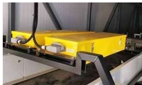
PI-MSKA system mounted above conveyor belts
