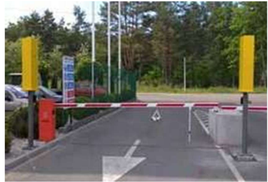
PI-MSKA system with two detectors positioned opposite each other
