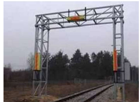
The PI-MSKA railway system with an upper detector and two detectors positioned opposite each other
